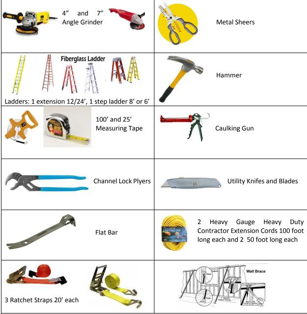
**Wall Bracing:** You will need some type of temporary wall bracing to use to align the wall until the roof panels are set and loaded. We can also use pieces of 3/4" emt conduit with flattened ends and drilled holes, for braces. We will need approximately 50 braces per kit.
